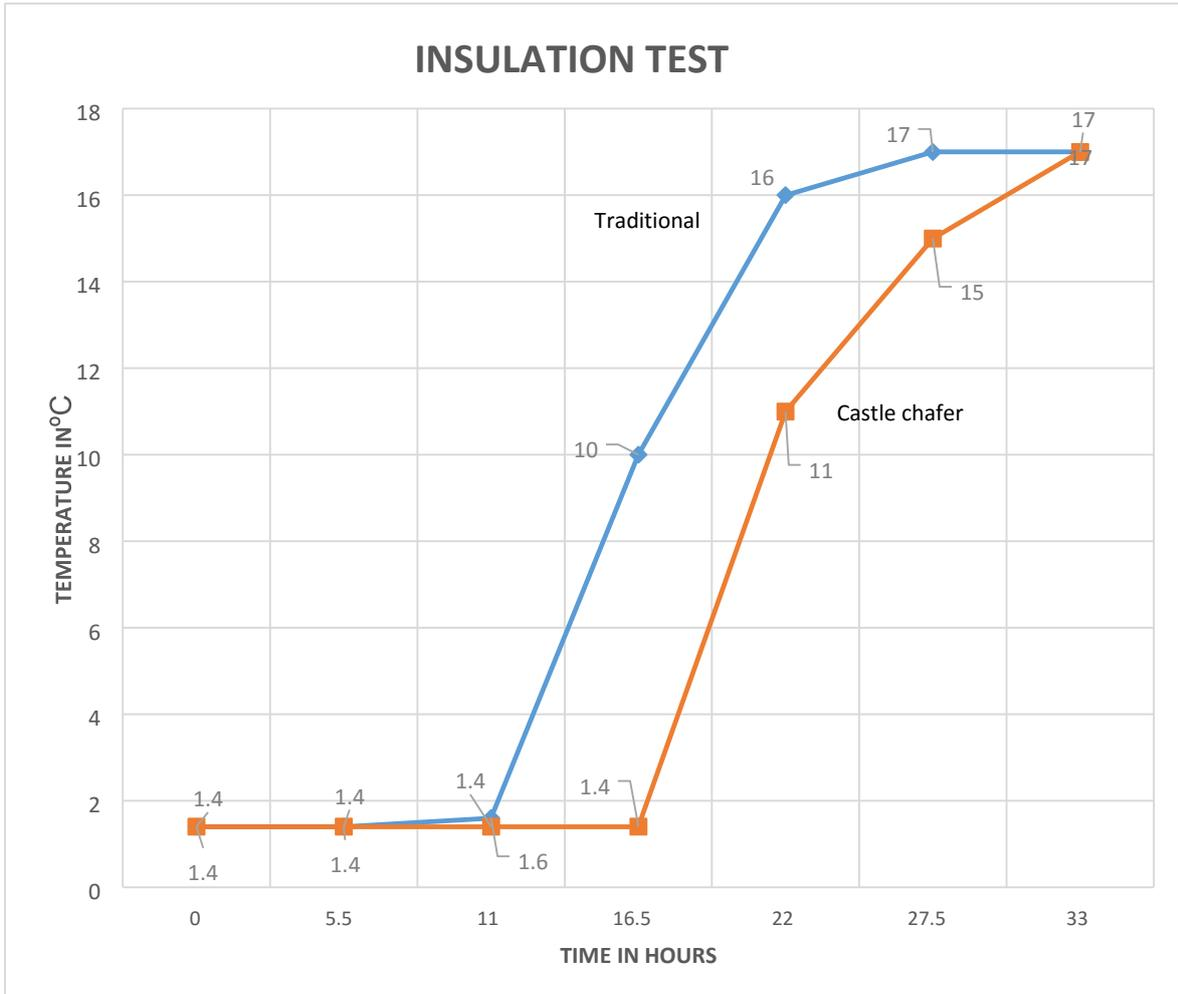
Test used 2 kilograms of ice
